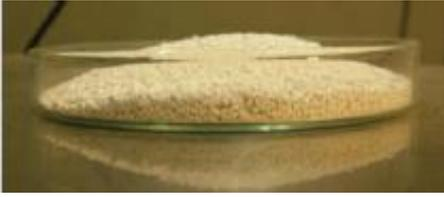
**Figure 39: CSH granules (Petzet and Cornel 2009).**
