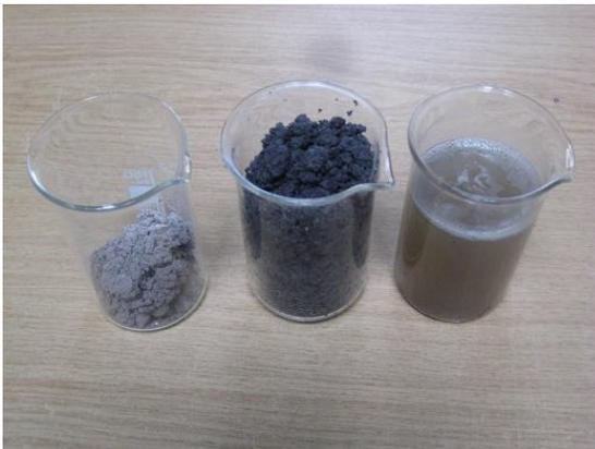
**Figure 37: Amorphous struvite from Seaborne process after atmospheric drying and after centrifuge separation, as well as the liquid phase from the centrifuge.**
