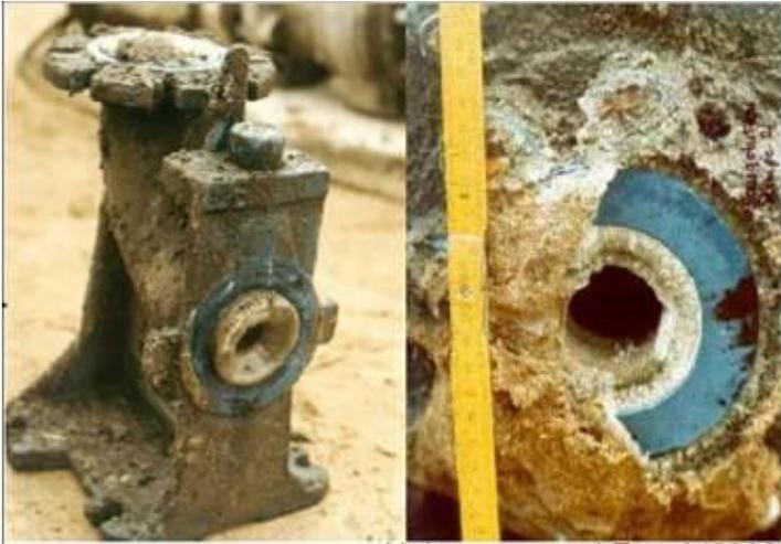
**Figure 23: A Pump and aperture with struvite incrustations (Heinzmann 2009).**
