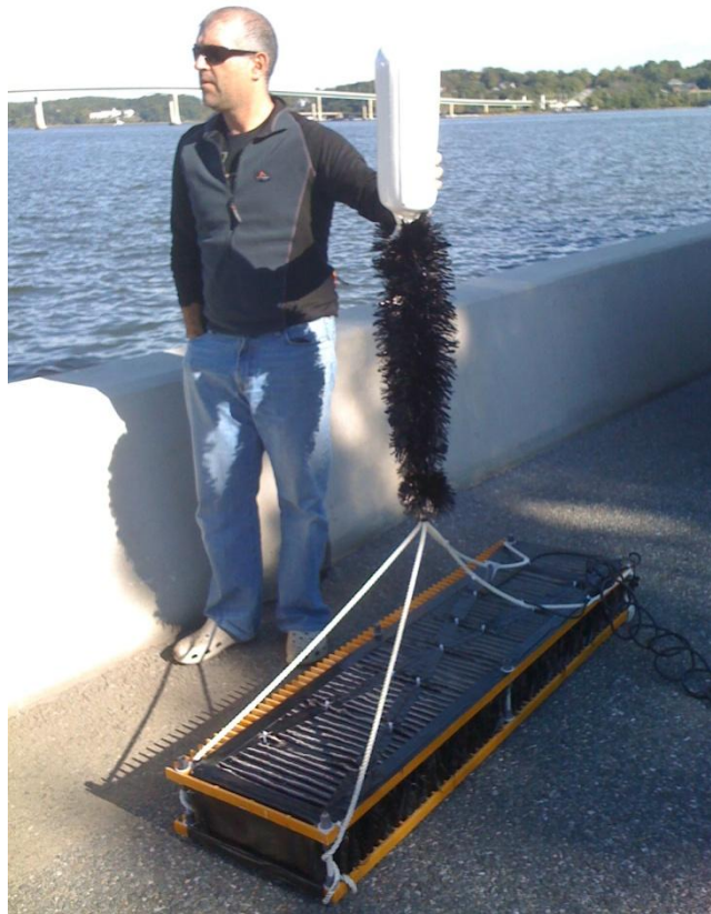
Figure 1. Leonard (Lenny) Tender standing next to a benthic MFC before deployment. Graphite plates (in the yellow casing) are deployed in the marine sediment with a graphite brush cathode in the overlaying water column.
