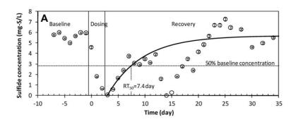
Proven in field trials to stop sulfide production
