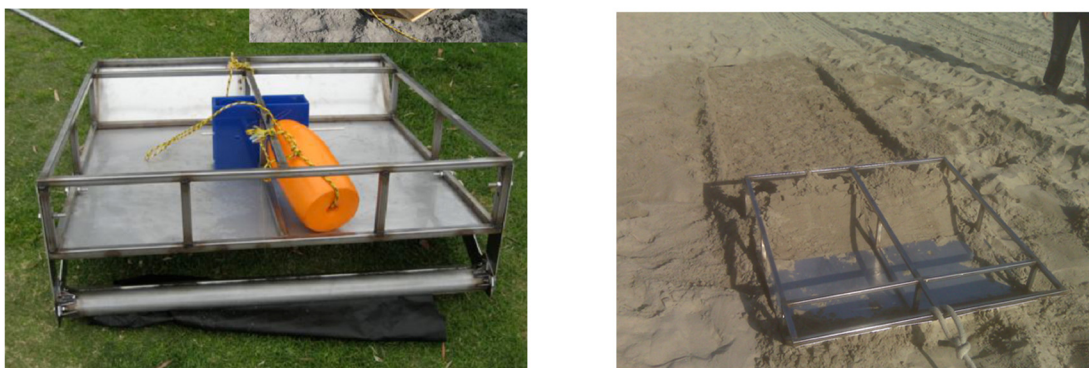
Fig. 5 – Photographs depicting “magic carpet” BMFC (provided by B. Chadwick, SPAWAR, San Diego). Left: embedment sled loaded with a rolled up carbon cloth anode. Right: deployment testing on beach, anode unrolled and buried beneath sand as sled is pulled forward. Sled detaches from anode and can be retrieved and reused.
